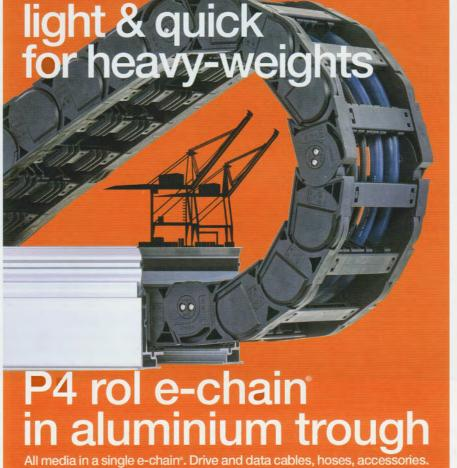
All media in a single e-chain<sup>®</sup>. Drive and data cables, hoses, accessories. Corrosion-free and resistant to salt water in the igus<sup>®</sup> aluminium trough. Saves 30% weight compared to steel troughs. Travel of up to 800 m and speed of up to 600 m/min with 57% less drive power. Moving energy made easy.
